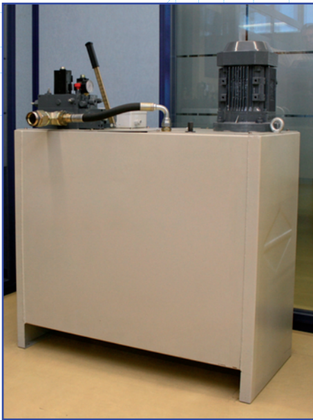
Figure 6. Re-Levelling with Auxiliar Motor
